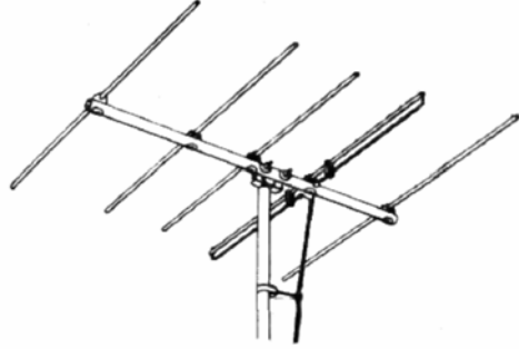
Figure 28.3: A Yagi-Uda antenna was invented by heuristics in 1926. The principal element of the antenna is the folded dipole with four times the radiation resistance of a half-wave dipole. When a wire dipole antenna is less than half a wavelength, it acts as a waveguide, or a director. When the wire antenna is slightly more than half a wavelength, it acts as a reflector [163]. Therefore, the antenna radiates predominantly in one direction (courtesy of Wikipedia [164]).
